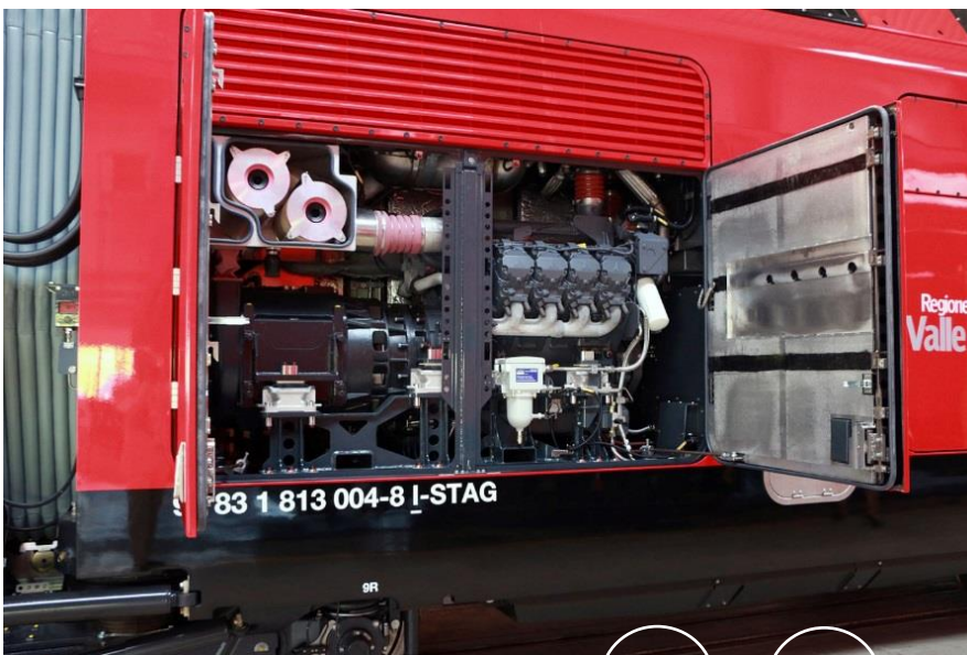
Figure 3-6: Stadler FLIRT Power Unit Access and Removal by Fork Lift Truck
