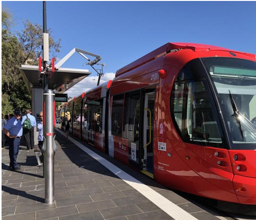
Figure 4-7. Example of Overhead Conductive Chargers for Rail
