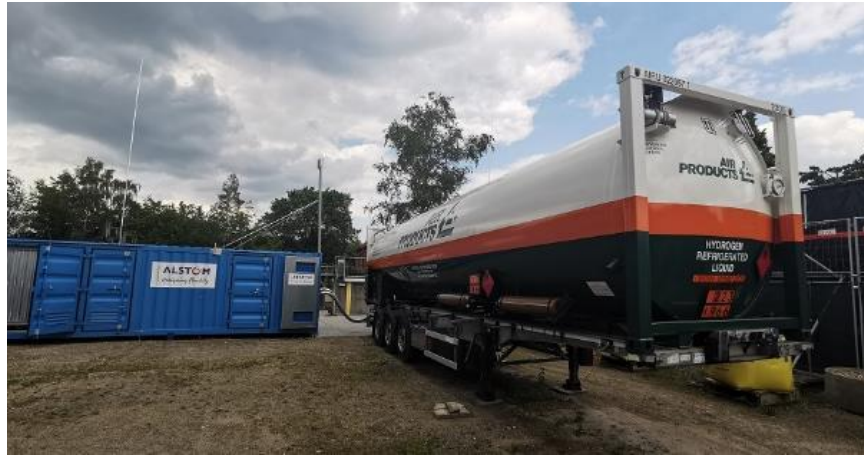
Figure 4-7: iLINT Mobile Refuelling Installation (Kent, 2019)
