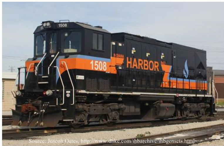
Figure 3-2: Indiana Harbor Belt CNG Switch Locomotive
