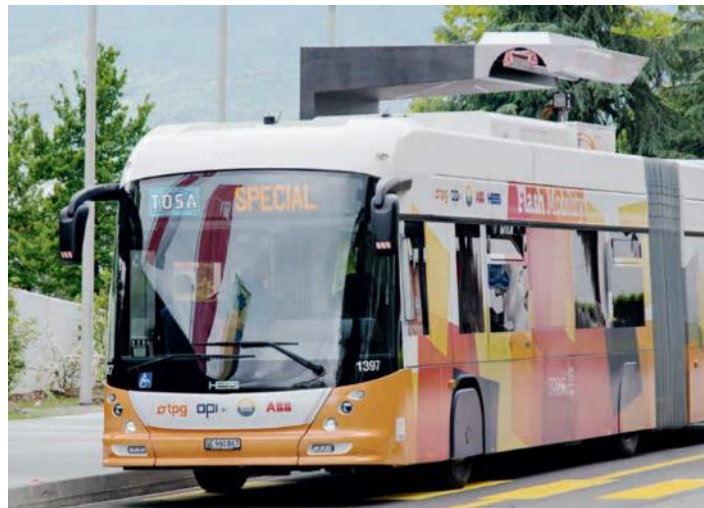
Figure 4-3: Rapid Charging Bus in Geneva (ABB Switzerland, 2016)
