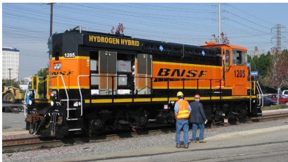
Figure 4-18: Hydrogen Fuel Cell Switcher (Hoffrichter, 2009)
