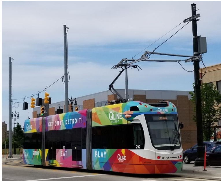
Figure 4-4: Battery-Powered Streetcar in Detroit at Charge Bar (Hoffrichter, 2018)
