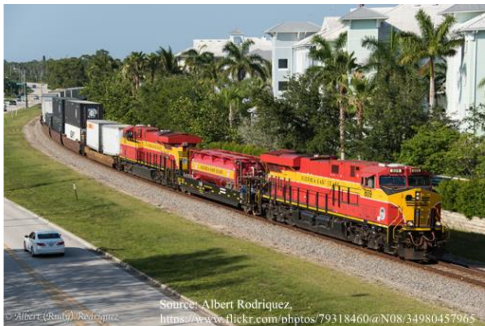
Figure 3-1: LNG Locomotives and Tender Car on the Florida East Coast Railway
