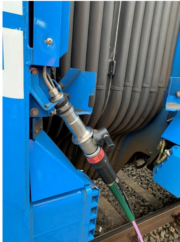
Figure 6-4: Hydrogen Refuelling Nozzle Connected to a Train (Hoffrichter, 2019)
