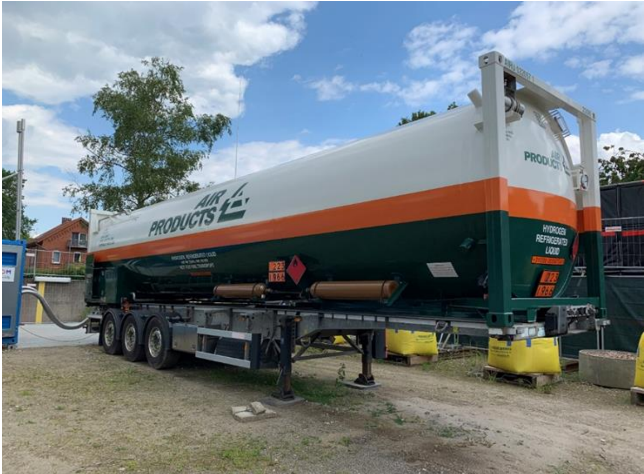
Figure 1 – Representative Temporary Hydrogen Storage Tank
