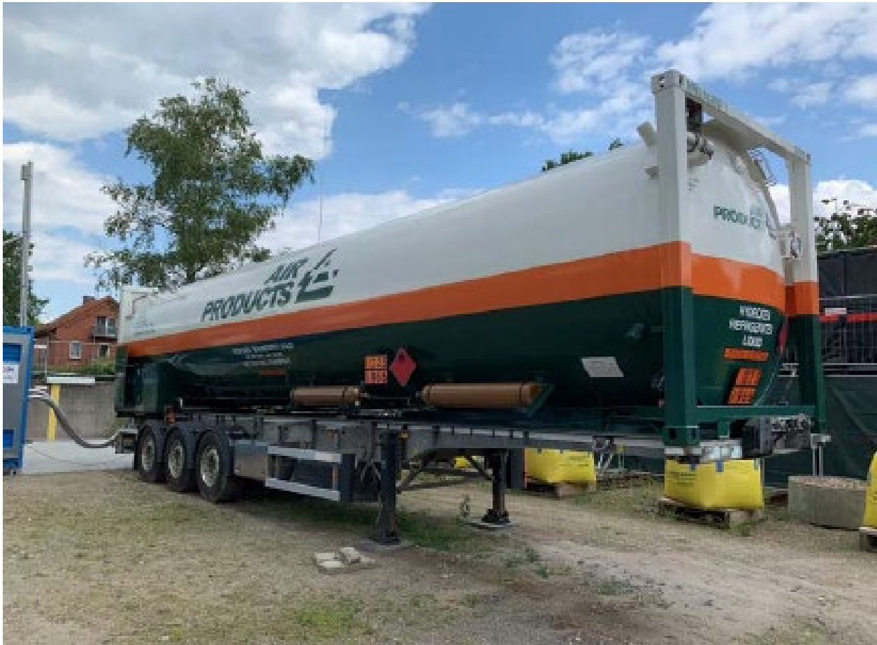
Figure 2-4. Example Hydrogen Fuel Storage Tank
