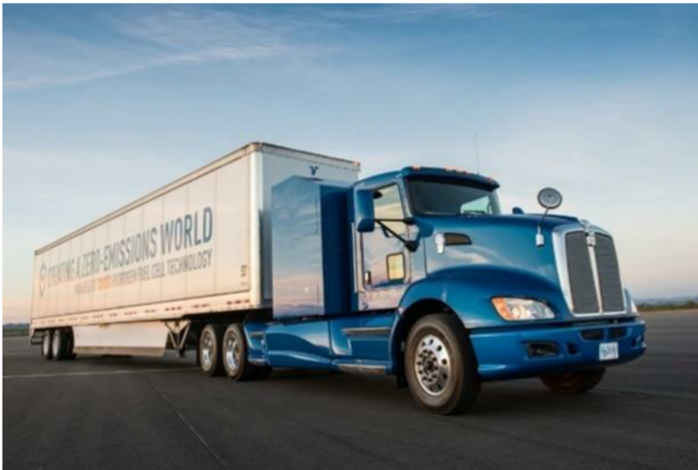
Figure 14: First generation Toyota Fuel Cell Semi Truck
