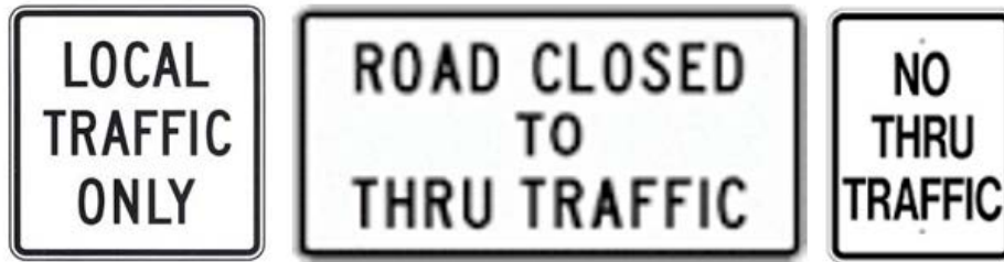
Figure 8-3: Local Access Signage Examples
