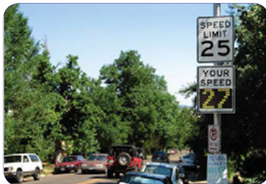
Speed feedback signs display a driver's speed as compared to the posted speed limit.
