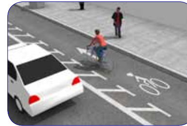
Buffered bike lanes can be accommodated along this corridor by narrowing travel lanes and removing the center turn lane.
