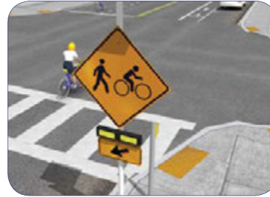
Rectangular rapid flashing beacons will increase driver compliance, providing more frequent crossing opportunities.
