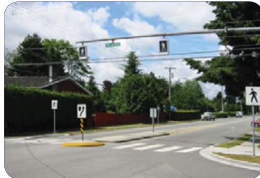
Median crossing islands allow pedestrians to focus on crossing one direction of traffic at a time.
