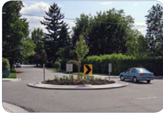
Traffic circles slow the flow of vehicular traffic into intersections.
