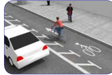
Buffered bike lanes will provide a more comfortable bicycling environment for bicyclists traveling between the Rancho Cucamonga Station and the proposed Deer Creek Channel and Day Creek Channel Trails.
