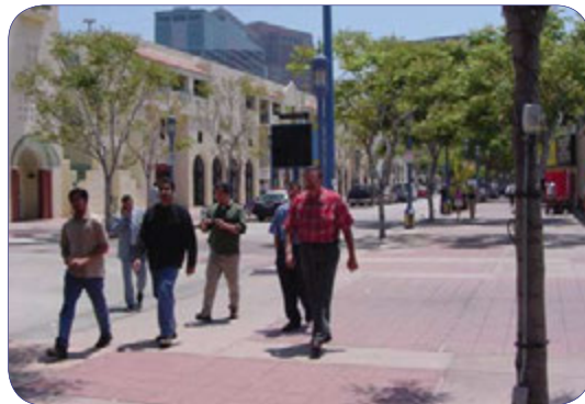
Sidewalks should be wider than four feet in areas with high pedestrian volumes.
