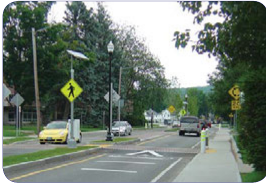
Crosswalks can be installed on speed tables to reduce speeds and make pedestrians more visible to drivers.
