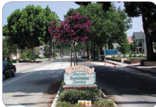
Landscaped medians lead to reduced speeds and create a more aesthetically pleasing streetscape.
