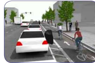
Stripe buffered bike lane to separate bicyclists from automobiles and to provide a more comfortable bicycling environment.
