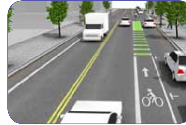
Coloration in the bike lanes should be used where drivers are likely to cross the bike lane to make a right turn.
