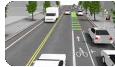
Coloration should be used in the bike lanes at the interstate ramps to enhance visibility of bicyclists in the bike lanes.
