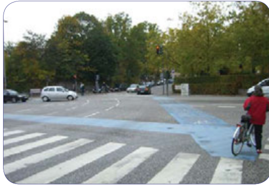
Intersection crossing markings help bicyclists with proper lane positioning.
