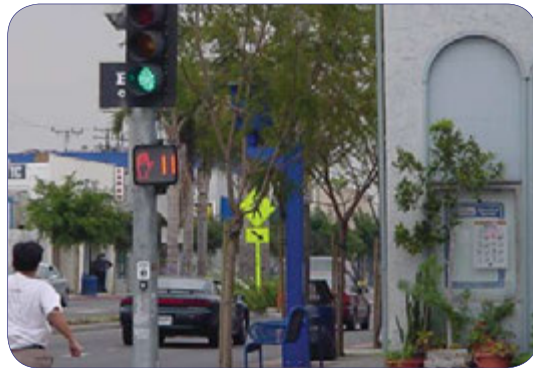
Pedestrian countdown signals display to pedestrians crossing the street how much time is left until the signal phase changes.
