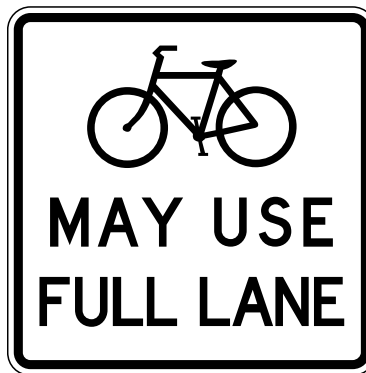
Figure 6.13 – Full Lane Shared Use Sign
