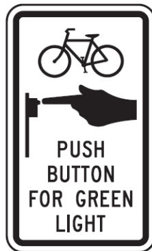
Figure 6.22 – Pushbutton Sign for Signals
