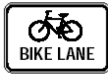
Figure 6.7 – Bike Lane Sign
