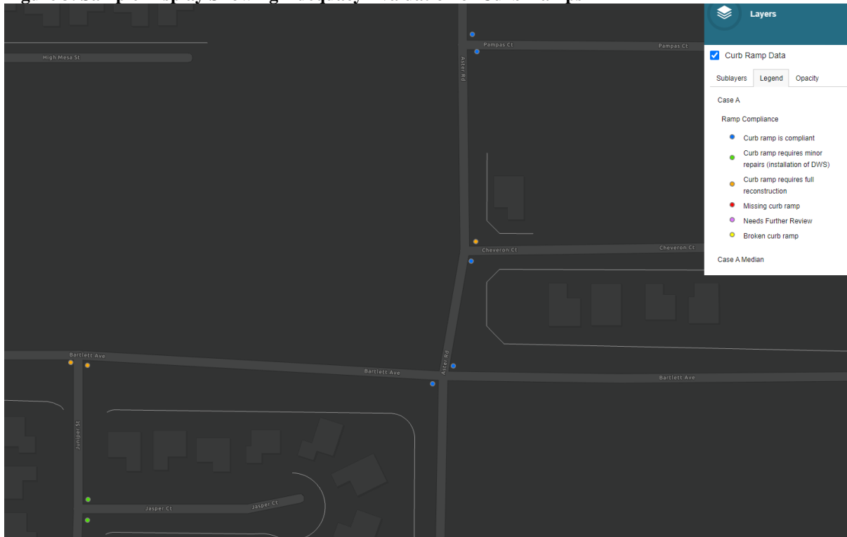
Figure 3. Sample Display Showing Adequacy Evaluation of Curb Ramps
